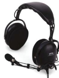
The heavy-duty over-the-head headset provides clear two-way radio communications in high noise environments. It has a certified noise reduction rating of 24 dB and includes a flexible noise-canceling boom microphone that fully rotates for left- or right-side positioning, cloth-covered ear seals, and in-line PTT. Cables are durable and flexible for demanding environments.
